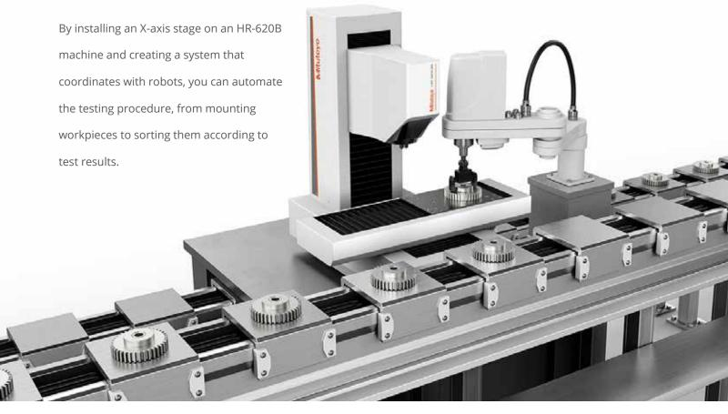
Example of Rockwell hardness testing machine automation on a production line
